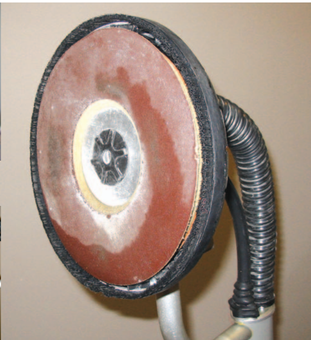
Figure 2. Shrouded ventilated rotary sander attached to vacuum.
