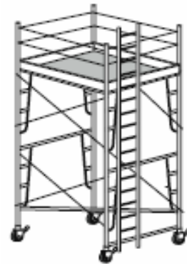
Example of a mobile scaffold with guardrail and mounting ladder (Source: OR-OSHA, 2005, Scaffolds: Temporary elevated work platforms ).
