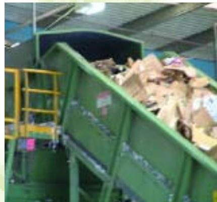
At the top of an inclined conveyor, material drops into the hopper and compaction chamber
