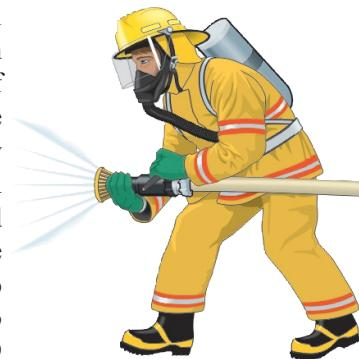
A pressure-demand or positive-pressure mode SCBA maintains a positive pressure inside the facepiece at all times. The system is designed to keep the admission valve open until enough pressure is built up to close it. Pressure builds up because air does not leave the system until exhalation. Internal facepiece pressure is always greater than external air pressure. Any leakage from the facepiece outward increases the protection.
