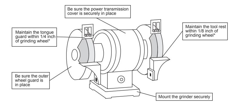
\* As the wheel wears down, readjust the tool rest and tongue guard. When you can no longer adjust them, replace the wheel.
