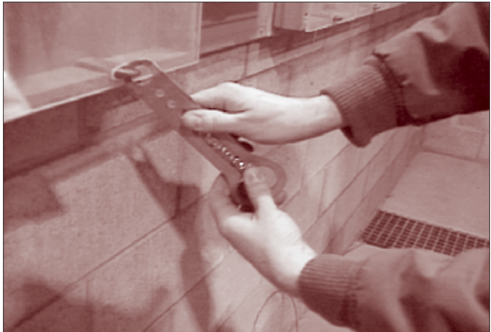
A positive sealing device has a seal that will show if the seal has been tampered with.
