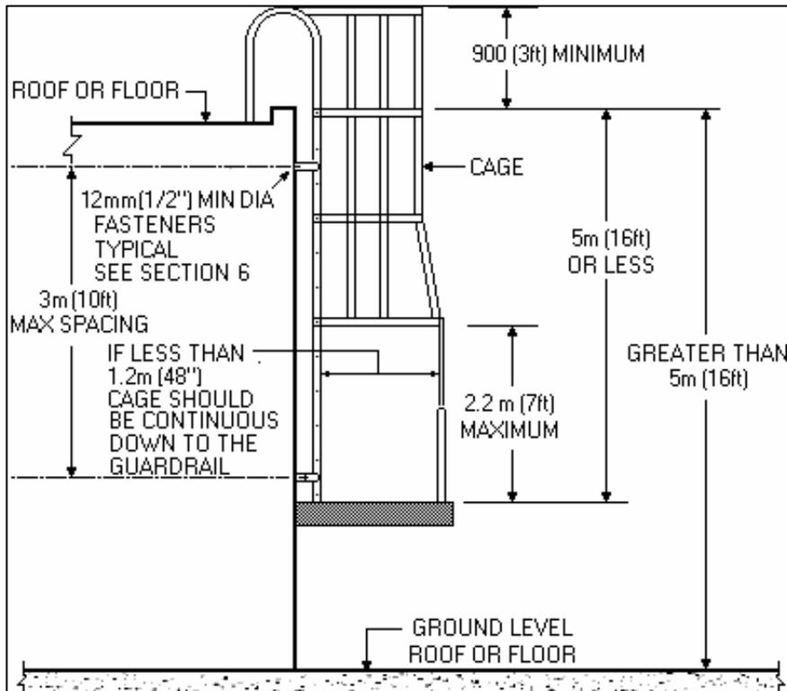
**FIG. 4: Typical Steel Access Ladder – Elevated Access**
