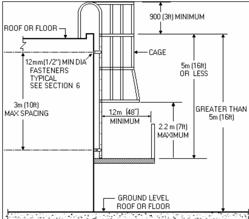
**FIG. 3: Typical Steel Access Ladder – Elevated Access**
