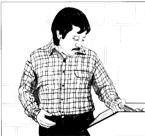
Tilted bins allow workers to remove materials from them without bending.
