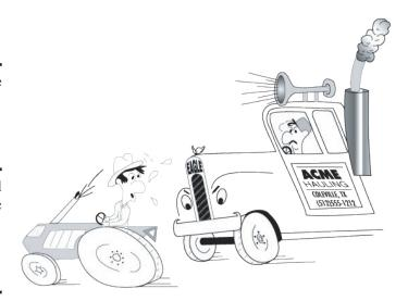
• Farm tractors and equipment require hazard-warning lights (flashers) when operating on public roads. White or amber flashers are mounted on the front, and red or amber on the rear. These lights must be activated when the vehicle is in operation.
