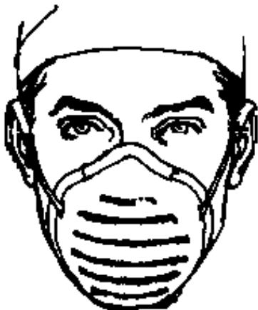
Dust Filter Mask: Traps particles out of the air.
